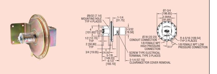
**Our highest precision** conventional large diaphragm pressure switch provides maximum dependability. In addition, it incorporates a visible set point indicator for maximum convenience. UL and CSA listed, FM approved for general service, these switches are suitable for most applications in air conditioning and industrial service. Electrical capability of 15 amps handles most small electrical loads.
