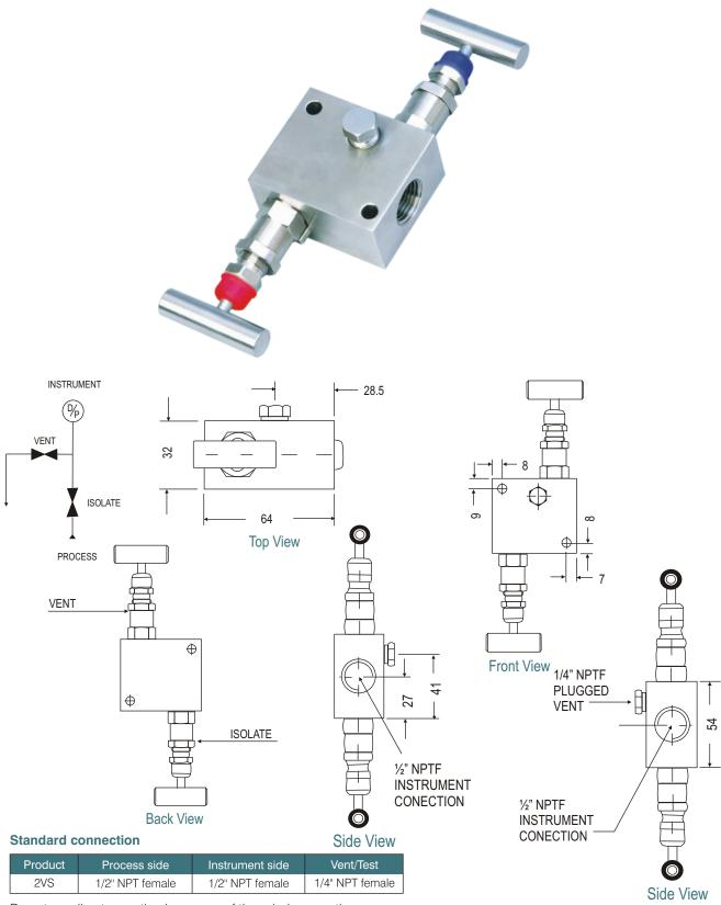
Remote or direct mounting by means of threaded connections.
