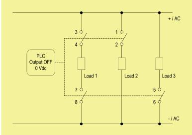
**Contacts 1-2:** Closing of contacts can be used for monitoring Contacts 3-4. No SIL Function.
