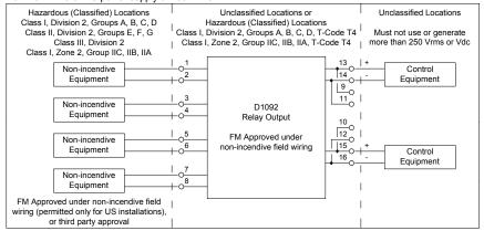
Non-incendive field wiring is not recognized by the Canadian Electrical Code, installation is permitted in the US only.
