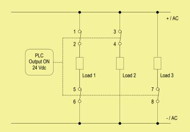
Contacts 1-2: SIL 3 Function is met when contacts are in open state.
