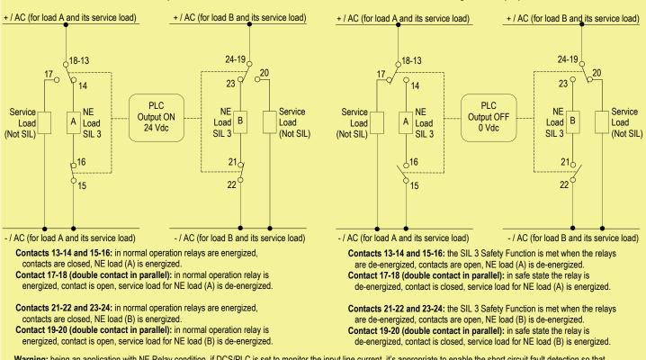
Warning: being an application with NE Relay condition, if DCS/PLC is set to monitor the input line current, it's appropriate to enable the short circuit fault detection so that DCS/PLC can detect short circuit fault of module (as, for example, the short circuit of a relay coil).
