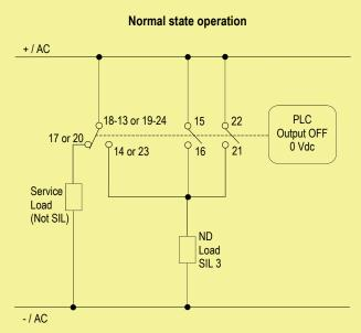
Contacts 13-14 or 23-24, 15-16, 21-22: in normal operation relays are de-energized, contacts are open, ND load is de-energized.
