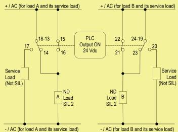
Contacts 13-14, 15-16: the SIL 2 Safety Function is met when the relays are energized, contacts are closed, ND load (A) is energized. Contact 17-18 (double contact in parallel): in safe state the relay is energized, contact is open, service load for ND load (A) is de-energized.
