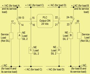
Contacts 13-14, 15-16, 21-22 and 23-24: in normal operation relays are energized, contacts are closed, NE loads (A, B, C and D) are energized.
