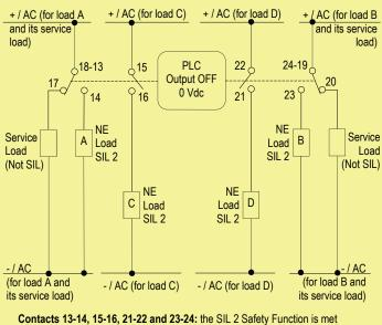
when the relays are de-energized, contacts are open, NE loads (A, B, C and D) are de-energized.
