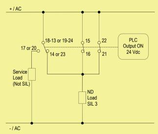
Contacts 13-14 or 23-24, 15-16, 21-22: the SIL 3 Safety Function is met when the relays are energized, contacts are closed, ND load is energized.
