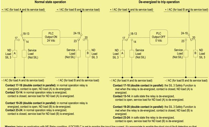
Warning: being an application with NE Relay condition, if DCS/PLC is set to monitor the input line current, it's appropriate to enable the short circuit fault detection so that DCS/PLC can detect short circuit fault of module (as, for example, the short circuit of a relay coil).
