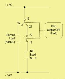
Contacts 13-21 and 14-22: the SIL 3 Safety Function is met when the relays are de-energized, contacts are open, NE load is de-energized. Contact 13-15: in safe state the relay is de-energized, contact is closed, service load for NE load is energized.
