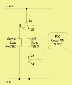
Contacts 13-21 and 14-22: in normal operation relays are energized, contacts are closed, NE load is energized.
