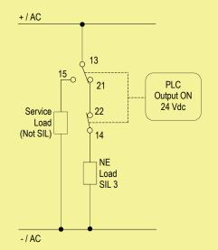
Contacts 13-21 and 14-22: in normal operation relays are energized, contacts are closed, NE load is energized. Contact 13-15: in normal operation relay is energized, contact is open,
