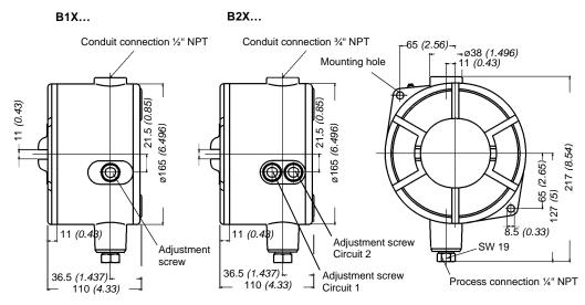
Fig. 10: Bourdon tube pressure switch type B1X .../B2X ...
