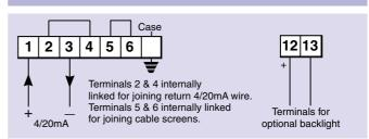
Calibrator Simulates 4 and 20mA input, selected by plug-
