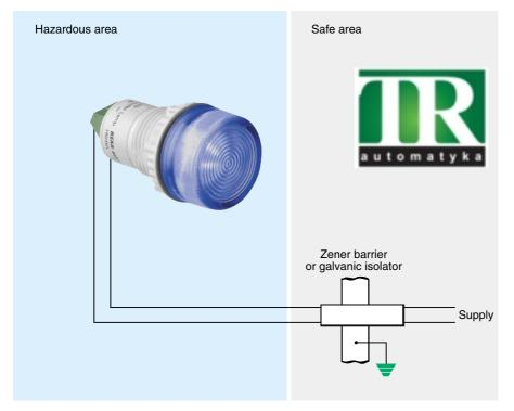
The BA390 cluster lamps provide reliable cost-effective visual status indication in all hazardous areas. Each BA390 contains a group of high efficiency light emitting diodes mounted behind a coloured diffuser to produce a bright, uniform output with a typical life greater than ten years. All models contain a 20mA current regulator which maintains constant brilliance and provides protection against excess voltages.
