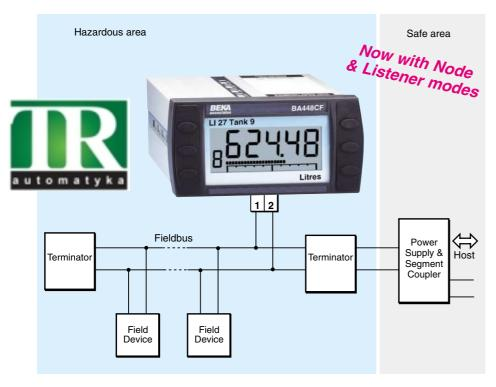
The BA448CF-F Fieldbus Indicator is an intrinsically safe instrument that can display up to eight fieldbus process variables within a hazardous area. A numeric annunciator on the left hand side of the screen shows which variable is being displayed. This version of the instrument supports FOUNDATION ™ fieldbus protocol; for PROFIBUS PA systems an alternative version is available − please see the BA448CF-P PROFIBUS datasheet.
