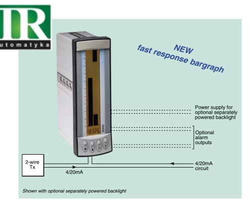
The BA526C is a new combined analogue and digital indicator which replaces the BA526. It offers enhanced features and improved visibility in a shorter enclosure. Like its predecessor, the BA526C displays the current flowing in a 4/20mA loop on a 100 segment bargraph and in accurate engineering units on a digital display. The instrument is loop powered but only introduces a 1V drop allowing it to be installed in series with almost any 4/20mA loop.
