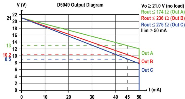
**Short circuit current:**  $\geq 50$  mA (55 mA typical).
