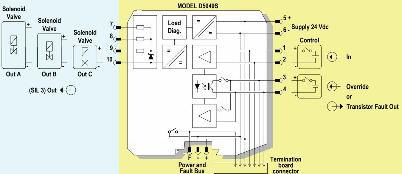
Terminals 3-4 dip-switch selectable for fault output signaling or override control
