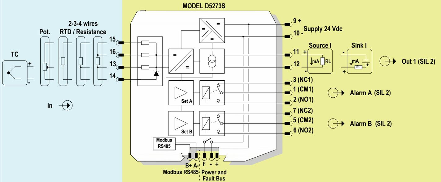
Application for D5273S , with 4-20 mA Analog Current Output
