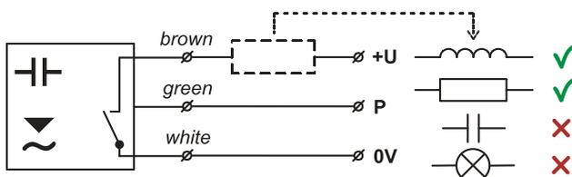
Note: In case of strong ambient electromagnetic interference, paralleling of conductors with power distribution, or for the distribution to distance over 30 m, we recommend to use shielded cable.
