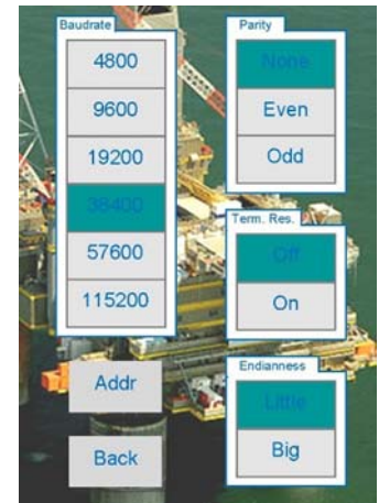
This image is shown when touching the "Modbus" cell in the set up menu screen. Here is possible to set Modbus communication parameters as baudrate, parity, terminal resistance, endianness and address, touching related cells.
