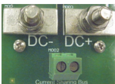
PSW1230 screw output terminals on copper bars: DC- is negative out pole, DC+ is positive out pole.
