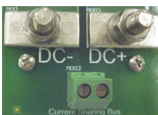
PSW1230 screw output terminals on copper bars: DC- is negative out pole, DC+ is positive out pole.
