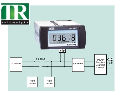
The BA618CF-F Fieldbus Indicator is a new cost-effective panel mounting instrument that displays a single fieldbus variable in a control room or process area. Housed in a robust panel mounting enclosure with an IP66 front, the instrument has a large, high contrast five digit display and a horizontal bargraph. The BA618CF-F indicator uses the same technology and compliments the well established BEKA eight variable fieldbus displays that are now in worldwide use.
